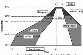
Average Ramp-Up Rate:3°C/second max. Ramp-Down Rate:6 °C /second max.
