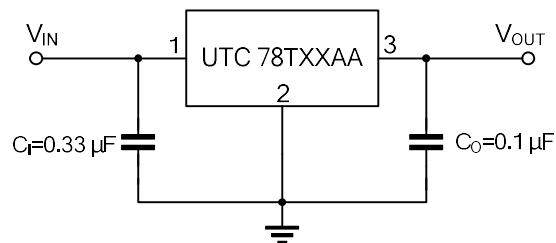
Note 1: To specify an output voltage, substitute voltage value for "XX".
